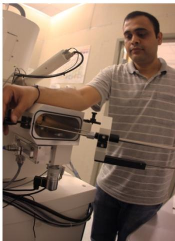
**Vinayak Bhat using the electron beam lithography instrumentation**
